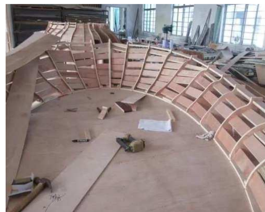
Figure 3. Wooden mold of prefabricated GRG module.
