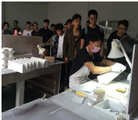
Figure 5. Modification and quality inspection GRG module.
